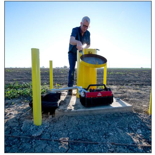
An engineering geologist with the California Department of Water Resources, measures groundwater levels at designated monitoring wells in Yolo County.
